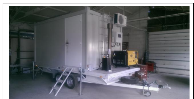
Figure no. 3, Mobile integrated surveillance system – assembly phase
